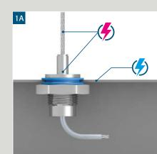
Continuously heightadjustable cable holder with central cable exit
