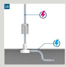
Continuously heightadjustable insulating holder with central cable exit
