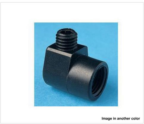
SEMKO certified cable gland for class II luminaires. They are supplied with the M7x1 threaded set screw removed. Maximum torque 130Ncm. For cables round hose H03VV-F from 4.8 to 6.5 mm in diameter and flat hose H03VVH2-F from 3x4.8 to 3.9x6.4mm in section.
